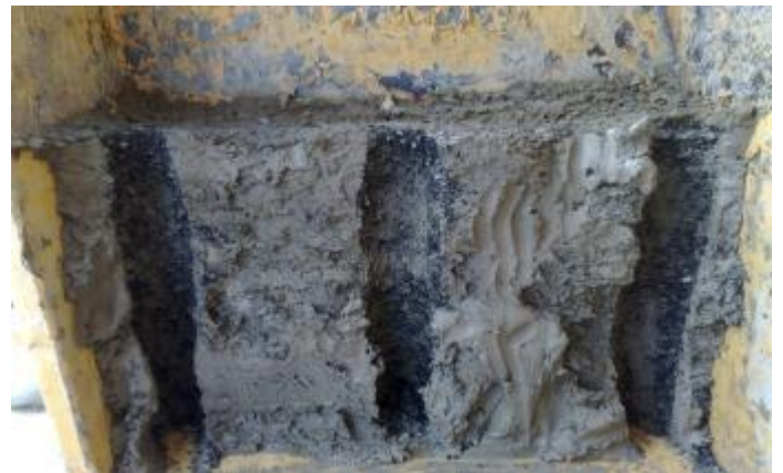
Plate 11. Stone columns failure ( S=3d , L/d=8 ).
