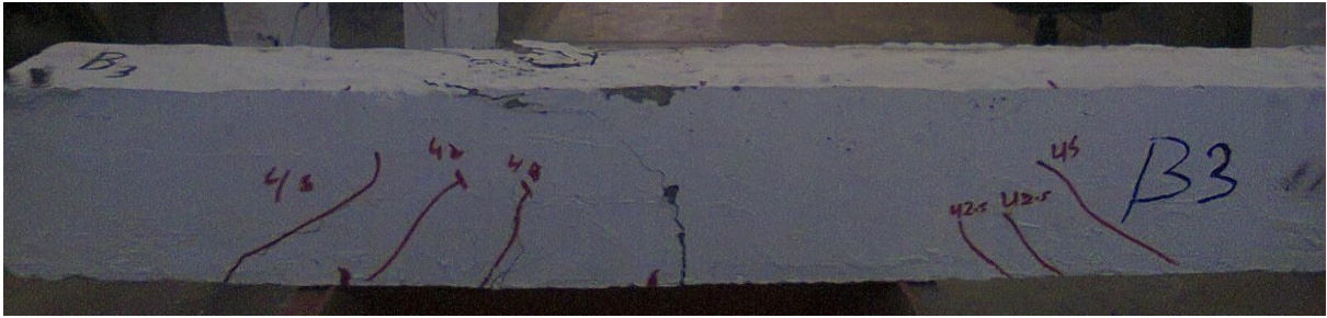
Figure 8. Crack patterns of beam (Hollow) B3.
