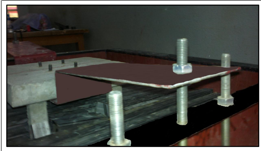
Plate 2. The pile foundation with the steel plate under the cap .
