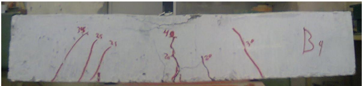
Figure 9. Crack patterns of beam (Hollow) B4.
