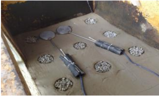
Plate 8. Configuration of patterns of stone columns, S= 3d .
