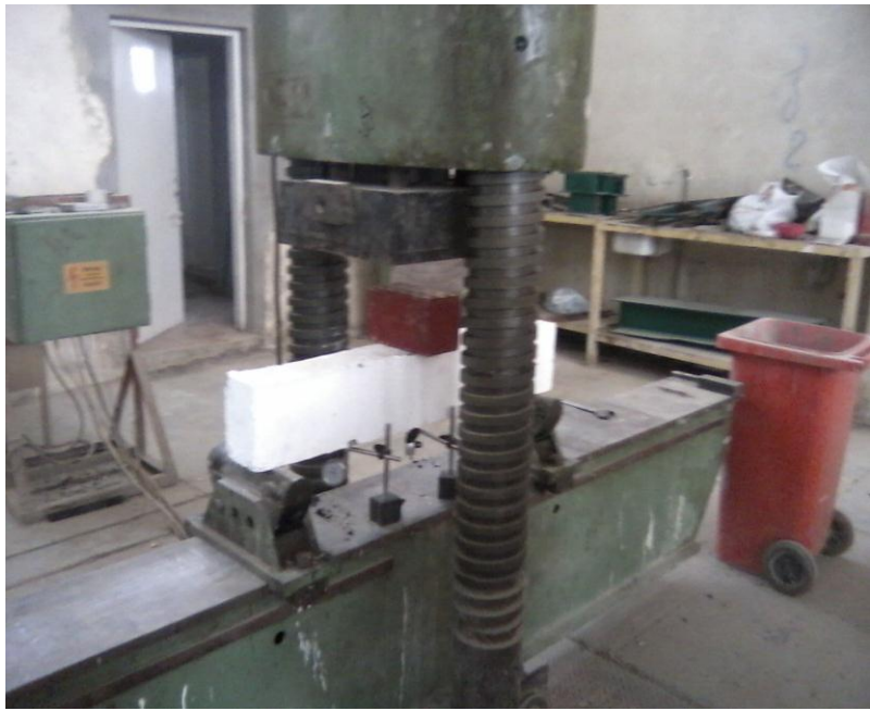
Figure 4. Beams under partial uniformly distributed loading.
