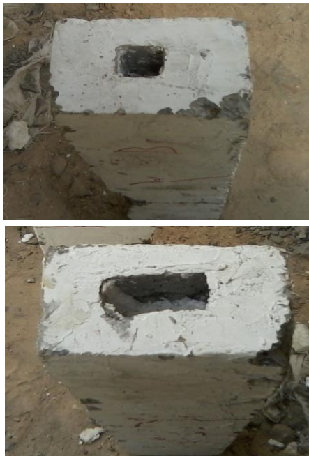
Figure 3. Recess through section of hollow beams.
